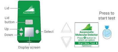
b. Wait for the detector to warm up (about a minute). Do not proceed until the detector displays the Prepare Sample Screen.
