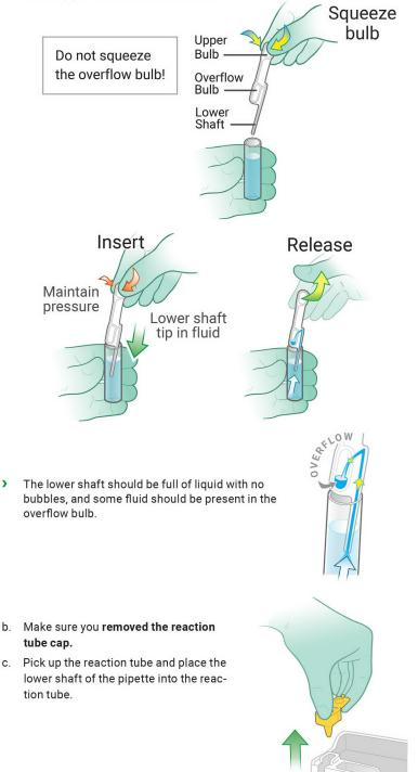
d. Fully insert the pipette, pushing down all the way until the overflow bulb rests on the edge of the reaction tube and the shaft tip is visible above the pellet.
