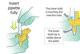
e. Firmly squeeze the upper bulb once, releasing the solution that is in the shaft. None of the fluid will come out of the overflow bulb of the pipette. It is normal for extra solution to remain in the overflow bulb. Do not squeeze the overflow bulb of the pipette or reuse any leftover solution.
