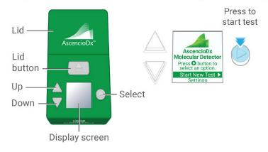
b. Wait for the detector to warm up (about a minute). Do not proceed until the detector displays the Prepare Sample screen.
