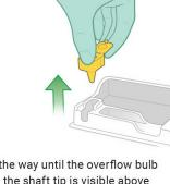
d. Fully insert the pipette, pushing down all the way until the overflow bulb rests on the edge of the reaction tube and the shaft tip is visible above the pellet.
