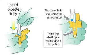
e. Firmly squeeze the upper bulb once, releasing the solution that is in the shaft. None of the fluid will come out of the overflow bulb of the pipette. It is normal for extra solution to remain in the overflow bulb. Do not squeeze the overflow bulb of the pipette or reuse any leftover solution.
